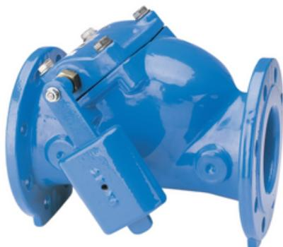
A swing check valve is a check valve in which the disc, the movable part to block the flow, swings on a hinge or trunnion, either onto the seat to block reverse flow or off the seat to allow forward flow.
