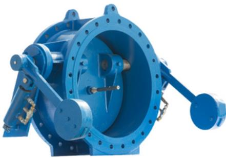
The tilting disc check valves are made of 2 piece body, designed to accomplish full flow opening by having the disc pivot or tilt in the flow media. The opening stroke range is much less than that of the conventional swing check valves, therefore reduces opening and closing time critical to controlling flow reversal and reducing water hammer. The full flow area with lower headless ensure valve will operate with the highest efficiency and durability.
